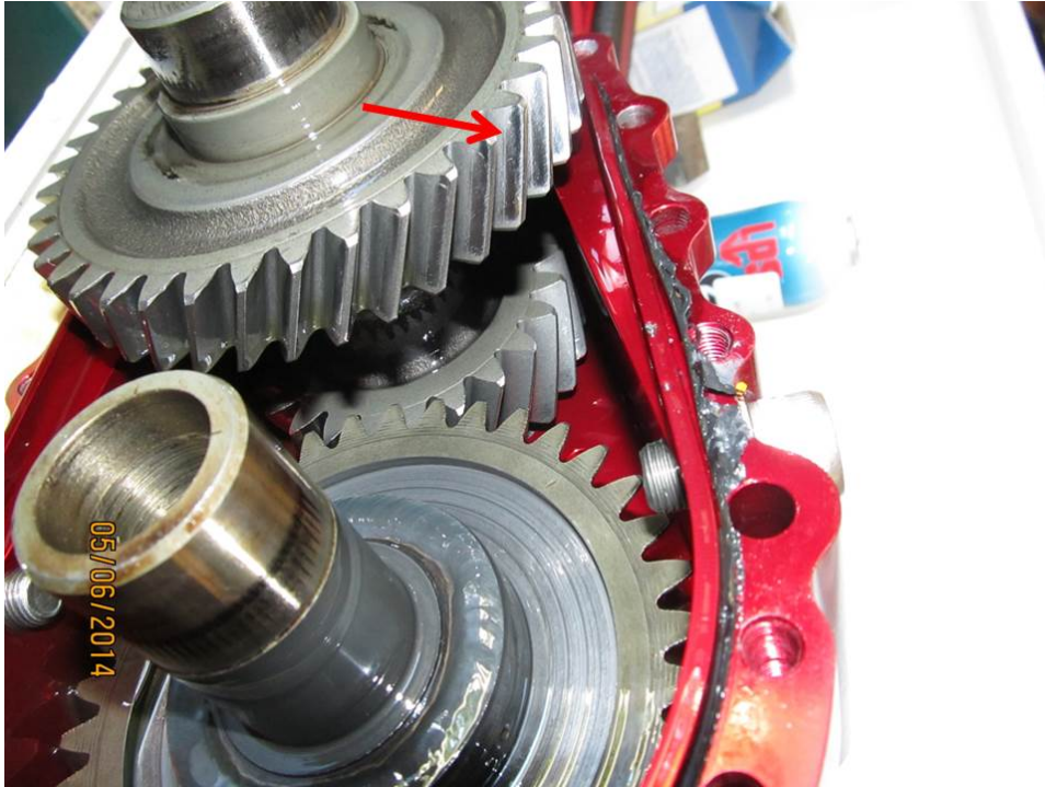
Photo 16 - Arrow shows polished area of wear.
