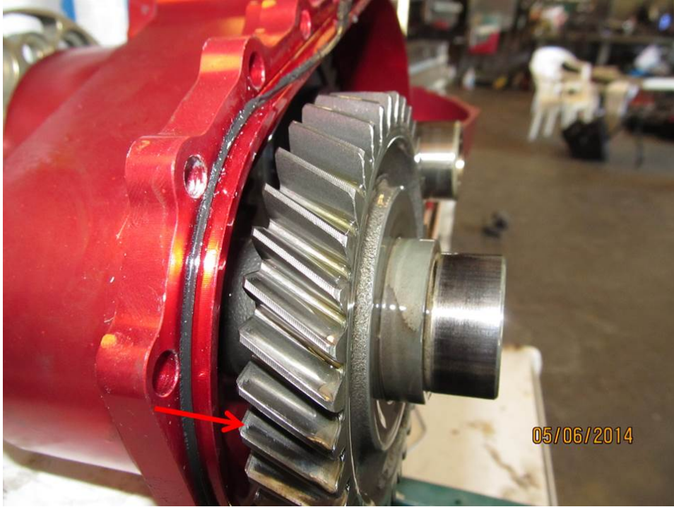
Photo 15 - Arrow shows polished area of wear.
