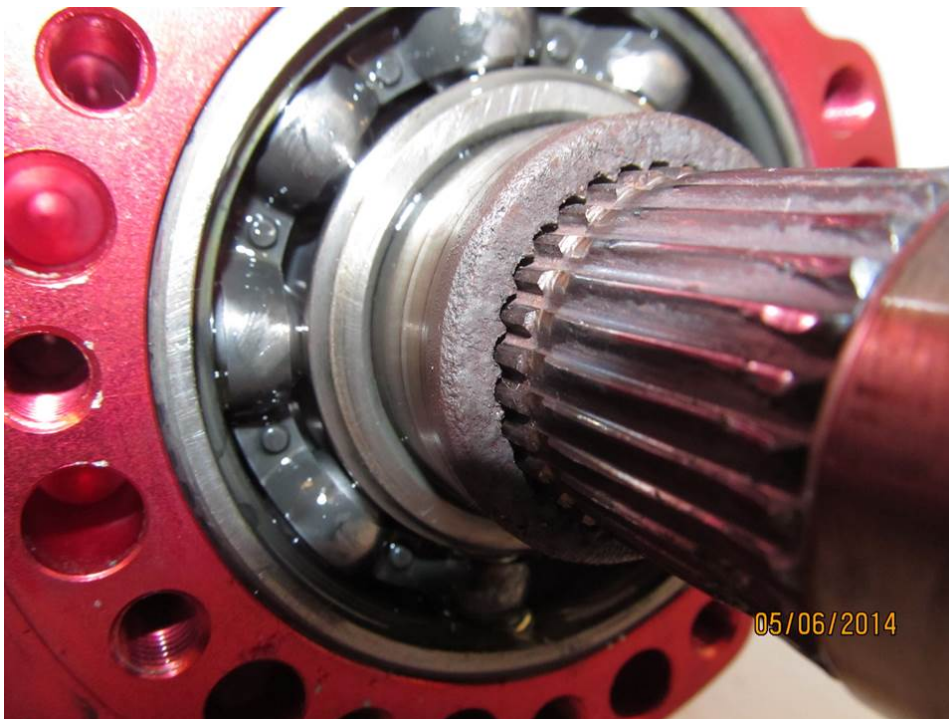
Photo 18- The spline shaft is pushed to the right, opening the gap between the PSRU input spline and the spline shaft.
