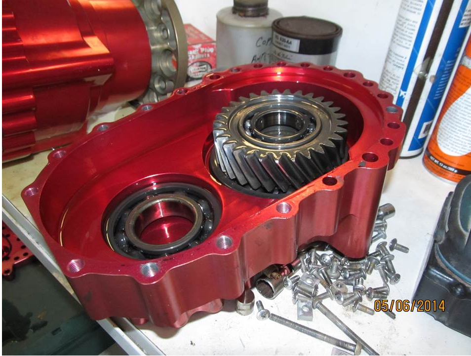
Photo 13 – PSRU opened. The oil in the case appeared clear. There was no sediment inside the case.
