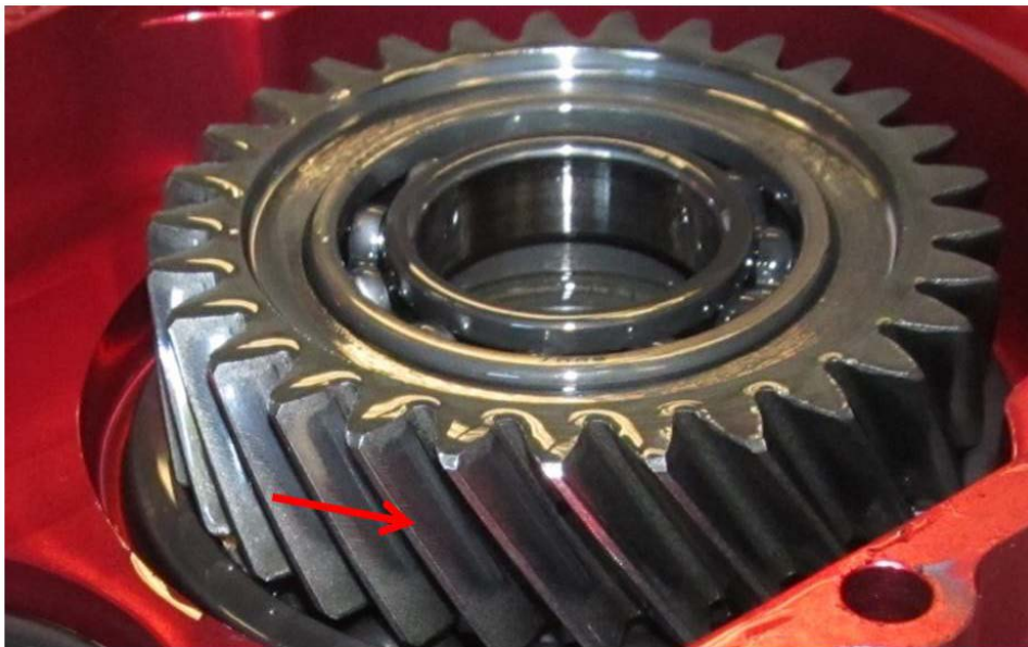
Photo 14 – Arrow shows polished area of wear.
