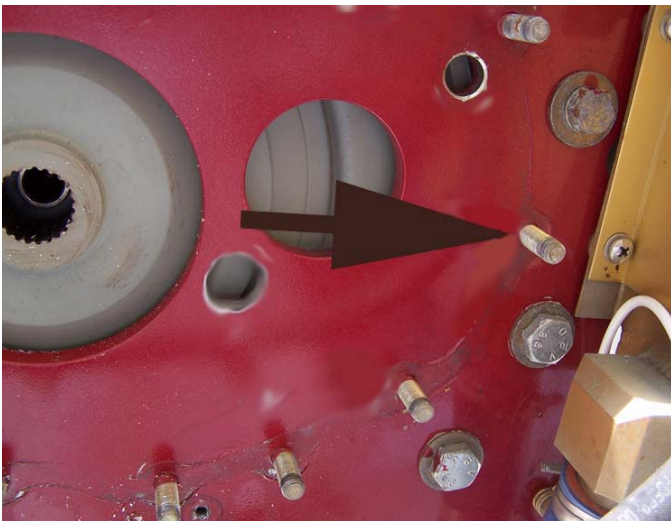
Arrow shows stud to cut off.
