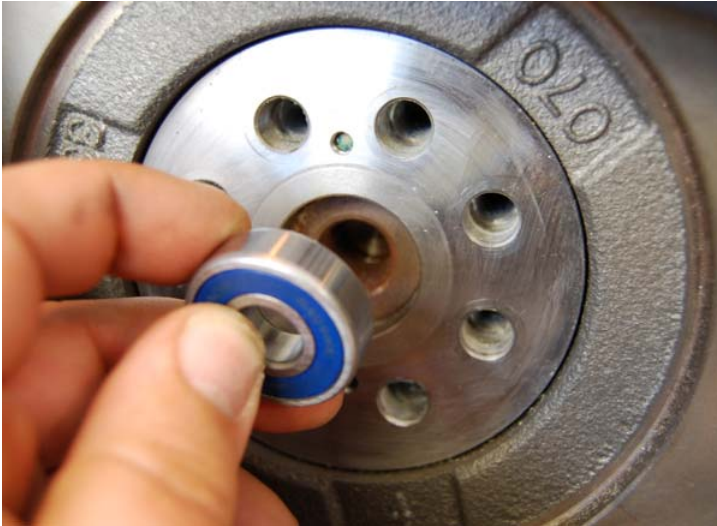
Inserting the bearing
