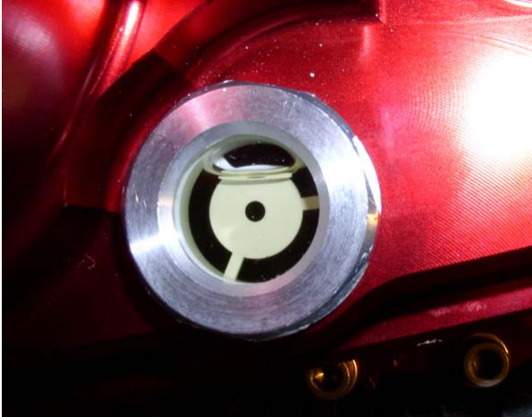
Proper fill level indication when level.
