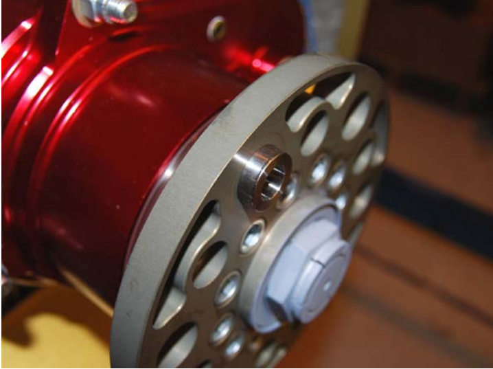
Fully seated long MT bushing
