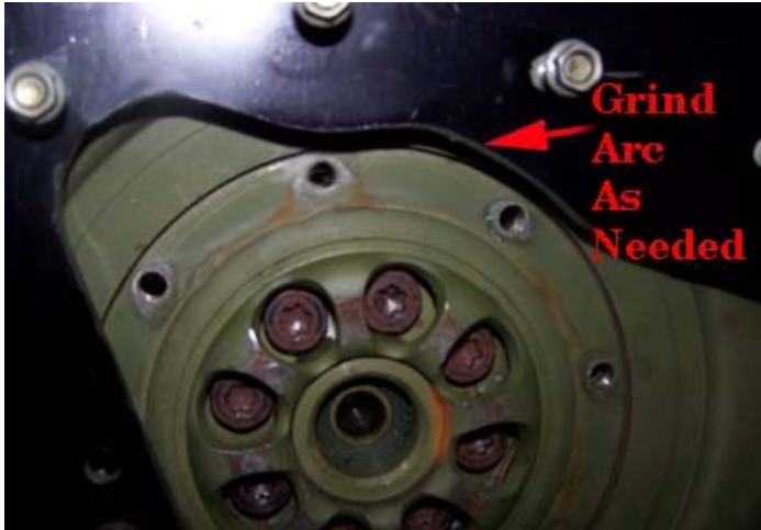
Arc ground in plate.
