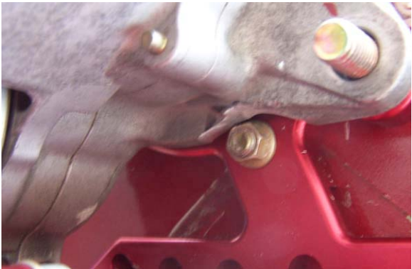
Interference between nut and starter.
