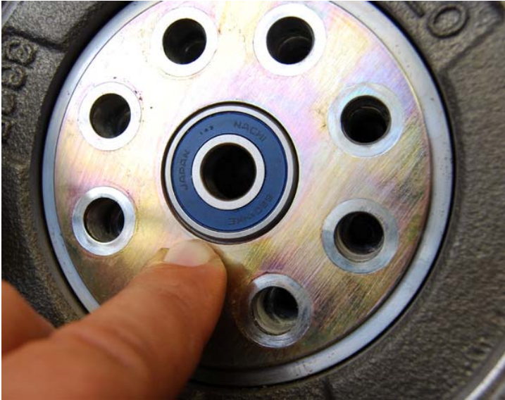
Proper bearing height
