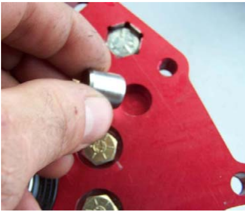
Inserting the alignment pins
