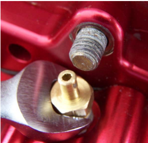
Vent Fitting (MUST REMAIN CLEAR)
