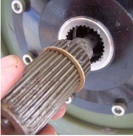
Inserting the spline shaft.
