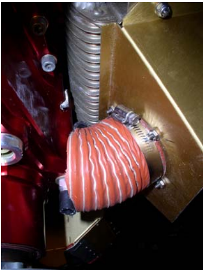
Radiator shroud blast tube.
