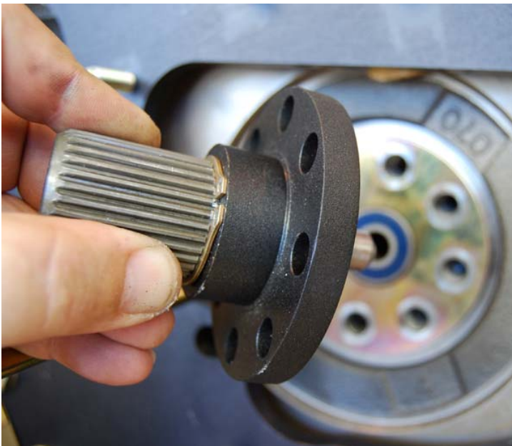
Shaft in adapter disk first.
