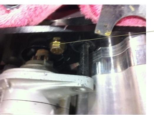
This mount bolt will get cut Out when the starter hole is enlarged, also you might have to grind the ears a bit for clearance
