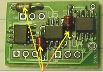
have been upgraded but everyone should check their SDS ECU. Zener diodes are shown on the upgraded board to the right so you know what they look like. It seems that perhaps inductive spikes from the engine starter motor may be damaging some of the driver chips.
