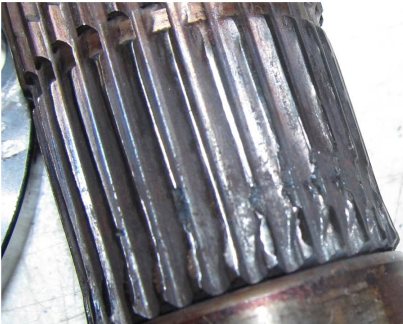
Photo 2 – Engine end of the spline shaft - The thicknesses of the spline teeth on the engine end of the spline shaft were reduced by more than 75% due to wear. The remaining thinned-edges of the spline teeth were bent over due to rotation of the spline shaft within the drive disk adapter.
