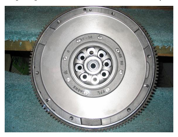
Back side of flywheel. The pulled side of the rivet is hidden by the small caps.
