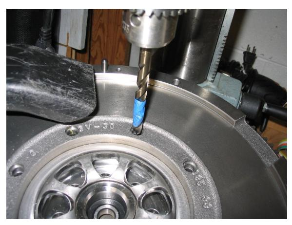
Place the flywheel on two boards such that the rivet can escape the back side when punched out. This was performed using a ¼ in pin punch (which I happened to purchase at Home Depot – Lowes didn't have it at my store). The picture below shows all other holes with the rivets already removed. Center the punch and use a solid/heavy hammer, keeping the punch as straight as possible. The rivet should punch out with just a few light to medium blows.
