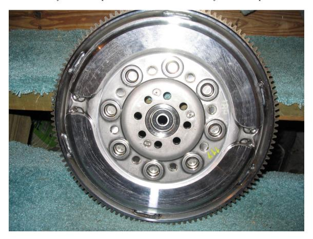
The flywheel profile. The side with the pins is the front side (this is the friction plate - my hand is on it)
