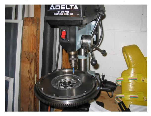
I used the following bits -1/8 and 5/16 inch cobalt split point for stainless and heavy steel. The bits cut through the material almost like it was butter (no cutting oil used). The drill press uses a slow revolution/speed, and I used light pressure - just enough to shave material.
