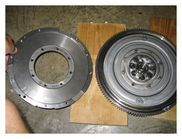
This is what the back side looks like where the rivet was punched through. You will note there is grease therein (which I assume is there for the sake of the spring torsion mechanism).
