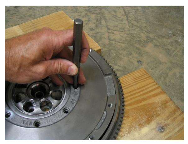
When you punch the last rivet the friction place will probably jar loose too. This picture shows it now removed (holding it). The flywheel holes are now ready to be tapped.
