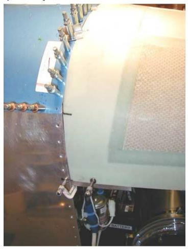
The final, and most critical cut is along the side seams. Here the top cowling is tucked inside the lower cowling and a sharp pencil is used to make the sanding line. Lots of block sanding will yield a perfect seam. Yes it can be done!
