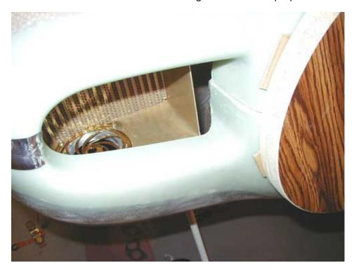
Fitting the rear seam works pretty much as it did for the lower cowling. Notice the black mark to help align it with the fuselage skin seam and the various clamps used to pull it tight. Take your time on this seam and get a good fit.
