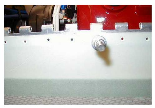
When drilling piano hinge, it is helpful to drill through both sides at the same time so the holes come out perfectly aligned. Note the piece of angle used to help hold the hinge plates parallel during drilling.
