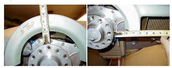
When you've got it just about perfect, you will notice that one or both of the oil cooler hose fittings may contact the bottom of the cowl. Ideally, they should just clear the cowl by about 1/16". You can locally remove ("core") a section of the honeycomb if needed to clear these fittings. I found that this was not required on my own installation. If you do core the honeycomb, lay a single layer of fiberglass mat over the cored area to reinforce it.
