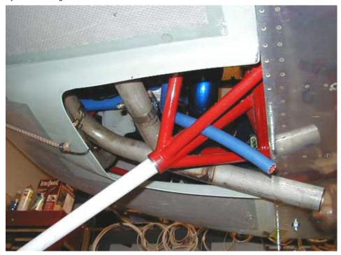
To this piece, I riveted a couple short hinge sections along the front edge. Note how my nose leg fairing cutout now starts at the front of the cowl flap instead of coming in from the rear of the cowling. To fit the leg fairing well, it had to taper to a point in the rear. On the inside I have riveted a small reinforcement plate around the slot. To remove the lower cowling, I pull the short hinge pin and drop the cowl flap away first. Then the main cowling drops down with no clearance problems.
