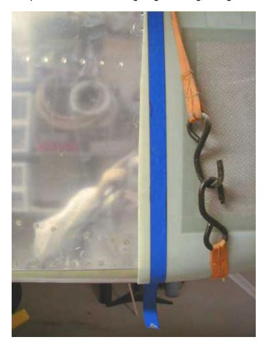
Once the marks have been made, remove the cowling and make your cuts with the Dremel cutting wheel. It is always best to cut just short of the mark and sand to the final fit. When sanding, use long strips of coarse sandpaper fastened to a long block of wood. It takes practice to make nice straight sanding strokes and establish a clean, straight edge. Have patience... Sand to the lines with plenty of test-fits as you go.
