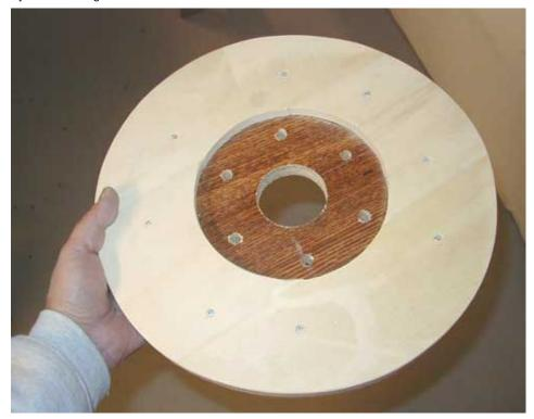
Start by tracing two 13.5" circles on a piece of 1/2" particle board or 1/2" plywood. Cut them out with a jig-saw or band-saw. Don't bother smoothing the edges just yet. You need two of these disks, one MUST be made from 1/2" material, the other can be thicker if you like. I used 3/4" particle board for the forward one, and 1/2" plywood for the rearward one.
