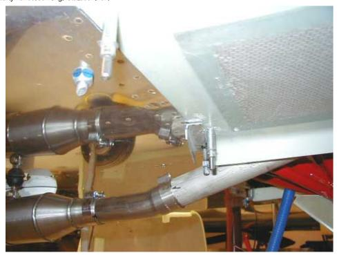
When you're finally satisfied, clamp it into position and mark the locations of your piano hinges or fasteners. You can install all of the lower cowling fasteners now if you choose. Consult the plans or vendor documentation for these procedures.
