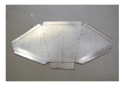
After cutting, bending, smoothing, and drilling, I made a lower attach bracket out of a piece of 0.5" angle and riveted it to the sides of the shroud. This gives me six points of attachment as well as forming a nice beveled intake.
