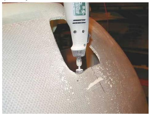
Obviously we need to do something about the honeycomb material and the now ragged edge. The best way to deal with this is to undercut the honeycomb layer with your Dremel and a cutting wheel. Be very careful not to cut into the thin fiberglass layers. The goal here is to slice away the honeycomb only so that you can pack the edges with filler.
