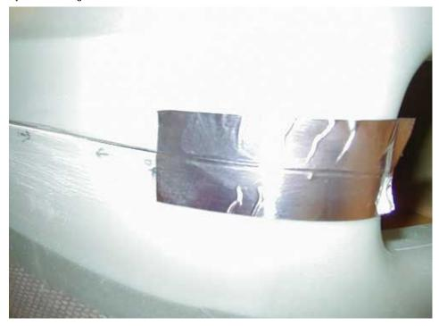
And the final fit! Note the cardboard wedges between the prop disk and cowl ring.
