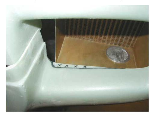
As you get closer to a good fit, use the wooden disk to make sure you have the cowling reasonably well centered. The following photos show that the inner fiberglass ring is 2.25" from the prop flange. Make sure you maintain this centered dimension, particularly as you start to trim the cowl to firewall seam.
