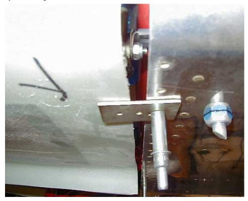
A Bungee cord hooked between the nosegear slot and somewhere on top of the motor helps to hold things up in front.
