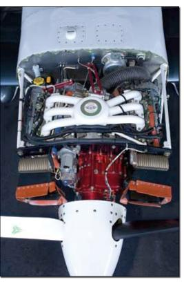
ing with a short break to install an Eggenfellner-recommended modification to the cooling system on my yet-to-be-run engine. The original design included two small side-mounted radiators with an oil cooler of approximately the same size mounted below the prop. These were all designed to fit within a minimally modified Van's IO-360 cowling.
