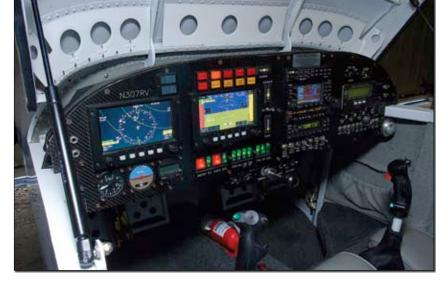
Twin Grand Rapids Horizon One EFIS displays are the centerpiece of Simpson's high-end panel. The data-logging capabilities of the system have been a huge help in refining the airplane.
