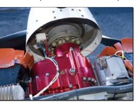
The Generation 3 PSRU, like its predecessors, is a two-shaft, four-gear arrangement meant to put the prop shaft on the same plane as the crankshaft.
