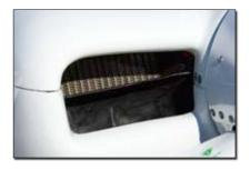
The horizontal duct borrows intake air from the copilot-side radiator and takes it back to the oil cooler. Precisely sizing and placing this splitter required many hours of trial-and-error testing.
