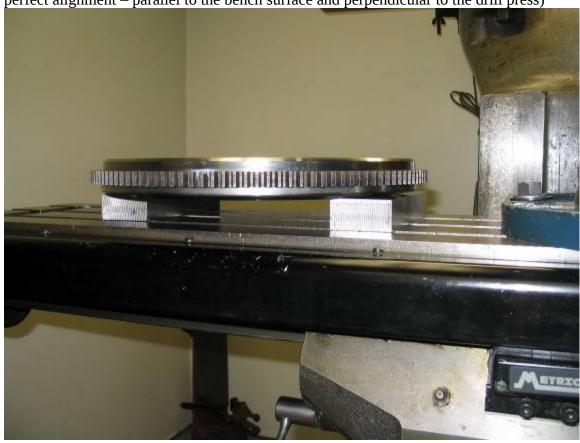
Next, in the picture below, the flywheel was clamped down. The point being that in your setup that you use some sort of clamp to keep the flywheel from moving while the tapping is performed.
