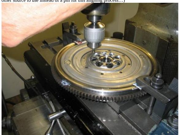
In the picture below the pin has been removed and the tap bit inserted, greased applied to help hold any metal chips. The drilling is performed at a very, very slow revolution. Once the first part of tap grips the material and cuts several threads within the hole it should continue to tap on its own (that is, let loose of the drill press handle and it should continue). Stop and reverse when the tap is made. Clean off the grease and the
