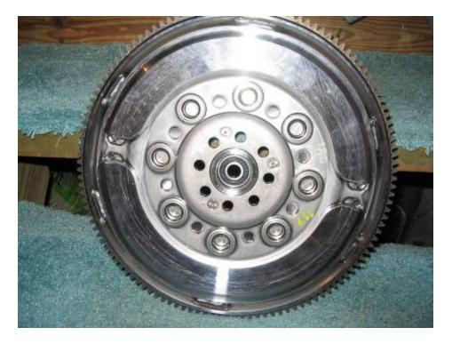
Back side of flywheel. The pulled side of the rivet is hidden by the small caps. In the picture above note that a few rivets and caps have been punched out (on the bottom).
