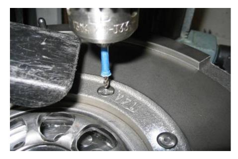
Using the existing rivet dimple I drilled first with a 1/8 in bit, no more than 15/32 inch deep. I marked this depth on the bit using tape. The black thing on the left is my vacuum nozzle. The picture above shows the 1/8 inch now drilled. The tape was bugged a little bit from shavings working their way up the bit.
