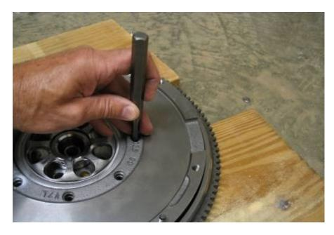
Place the flywheel on two boards such that the rivet can escape the back side when punched out. This was performed using a ¼ in pin punch (which I happened to purchase at Home Depot – Lowes didn't have it at my store). The picture above shows all other holes with the rivets already removed. Center the punch and use a solid/heavy hammer, keeping the punch as straight as possible. The rivet should punch out with just a few light to medium blows.
