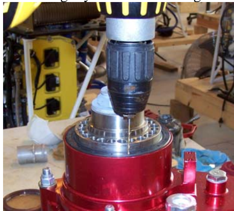
Carefully drill a hole in the old seal face.
