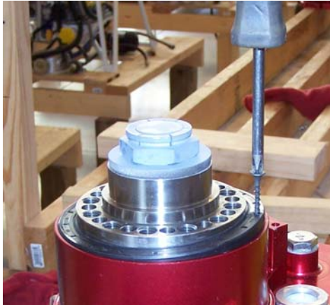
Using a jack-screw to raise the old seal.
