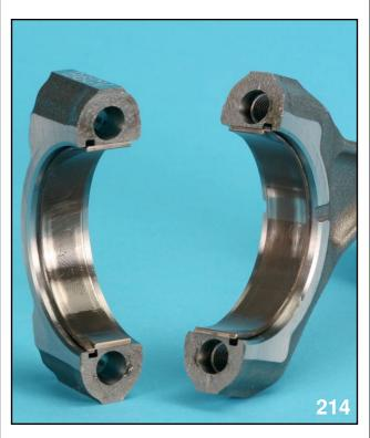
CONNECTING ROD CAP SEPARATED FROM ROD
