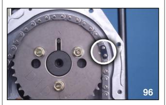
LEFT BANK INTAKE CAMSHAFT TIMING MARK
