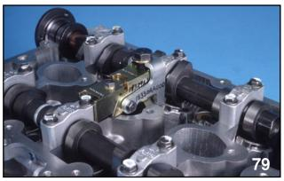
VALVE ADJUSTMENT TOOL PLACEMENT
