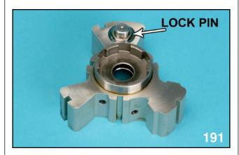
INNER ROTOR BUILT IN LOCK PIN
