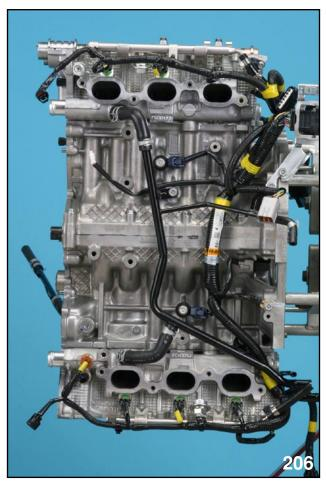
Wiring Harnesses, Coolant Lines and Hoses on Cylinder Heads
