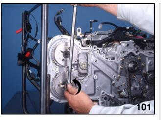
LOADING EXHAUST CAMSHAFT (RIGHT BANK)
