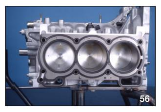
Cylinder Block with Head Gasket
