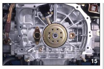
CRANK ANGLE SENSOR WITH RELUCTOR
