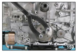
ST18355AA000 Pulley Wrench and ST18334AA000 Pin Set
