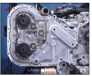
REMOVE CAMSHAFT SPROCKETS (RIGHT BANK)
