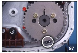
LEFT BANK EXHAUST CAMSHAFT TIMING MARK
