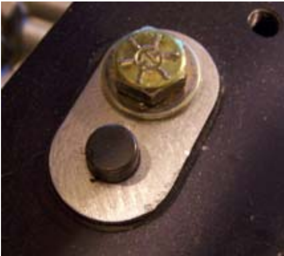
Index Plate over long dowel pin.
