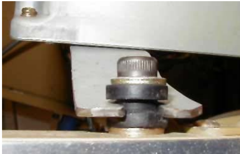
Close-up view of rubber shock mount on shoulder-bolt.
