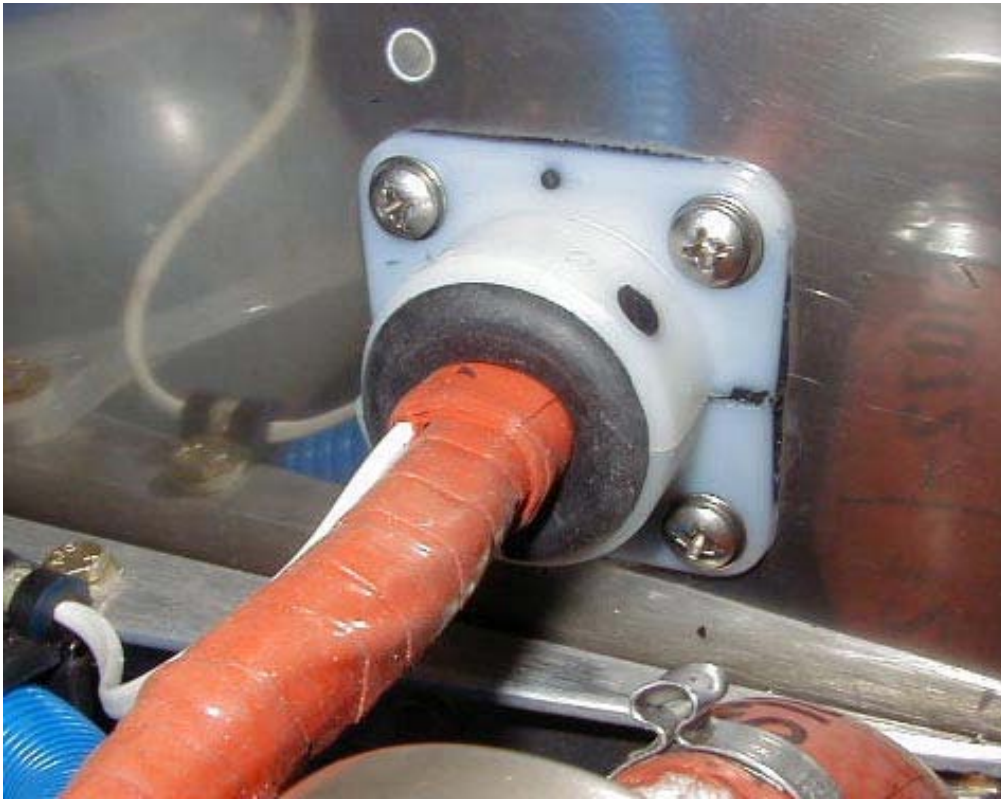
Aircraft Spruce p/n NMCS45A-11, Grommet p/n AN931-11-16 (you need 2 grommets)
